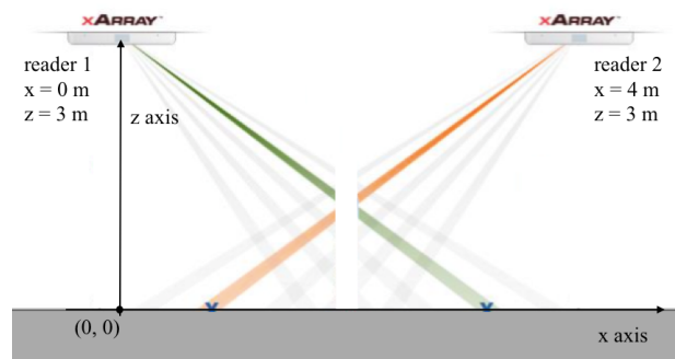
Figure 3: Impinj xArray installation set-up for data collection.
