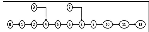
Figure 3 Precedence diagram of proposed Mixed Model
