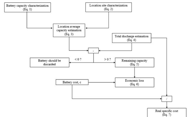
Figure 3. Method to classify batteries for smart meters
