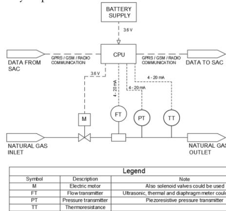
Figure 2. Schematic of NG meter with main components
