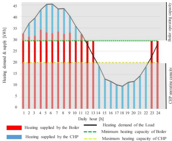
Figure 5. Supply of the load heating demand by the boiler and the CHP during an average day of March.
