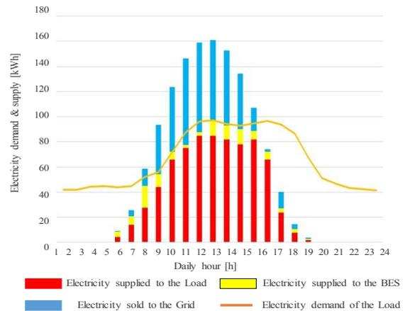
Figure 4. Dispatching of the electricity produced by the PV during an average day of July to the other PES modules.
