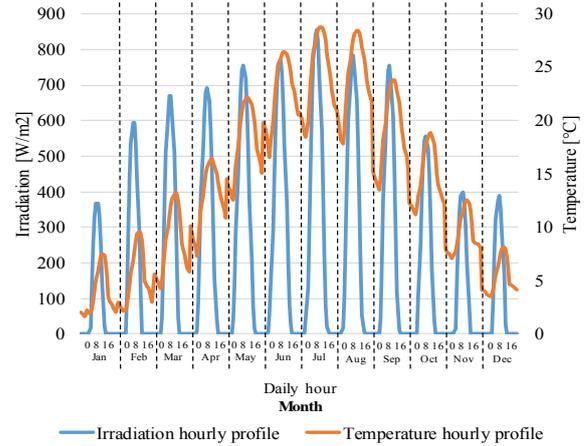
Figure 2. Irradiation and temperature hourly profiles of the installation site, for every month.
