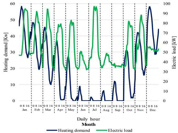
Figure 3. Hourly heating demand and electrical load of the user, for every month.
