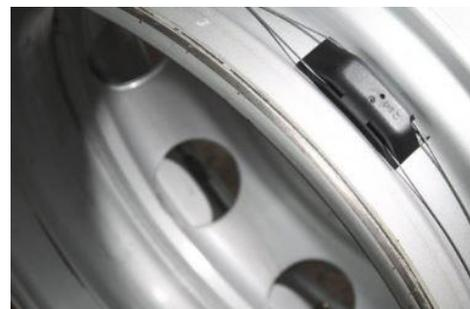
Figure 5: EFFIFUEL system developed by Michelin. It monitors some vehicle and tire parameters related to their condition, such as speed, temperature, pressure.
