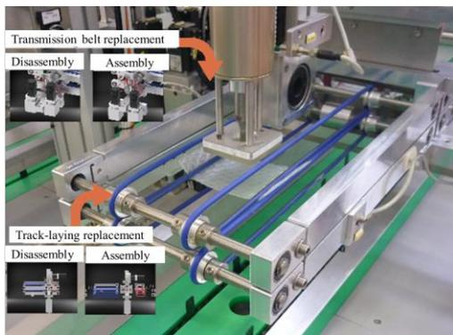
**Figure 6: visualisation through wearable devices of maintenance actions for restoring of an automatic packaging machines. Videos and virtual documents and instructions were elaborated by the authors.**
