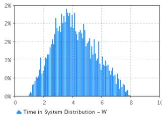
Figure 7: Probability distributions of the time in the system  $W$  for the uncoordinated charging process.
