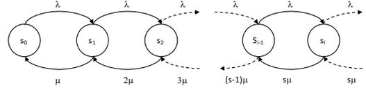
Figure 2: State transition diagram for the queuing model with an infinite population (M/M/s//∞).
