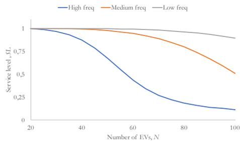
**Figure 6: Service level offered by of the charging process for the model M/M/s//N as a function of the number of EVs visiting the area considered (N) for each arrivals frequency considered.**
