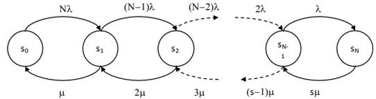
Figure 3: State transition diagram for the queuing model with a finite population (M/M/s//N).
