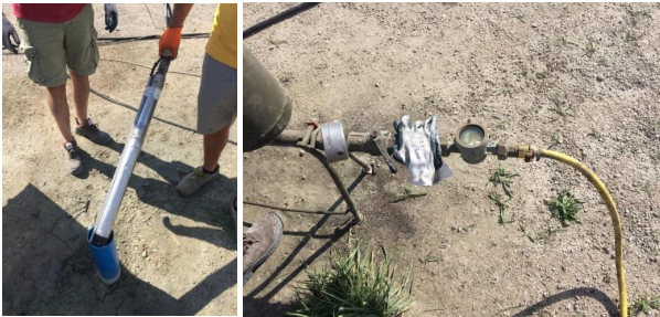
Figure 4: a) picture of the water pump and b) of the water volumetric flowrate meter.
