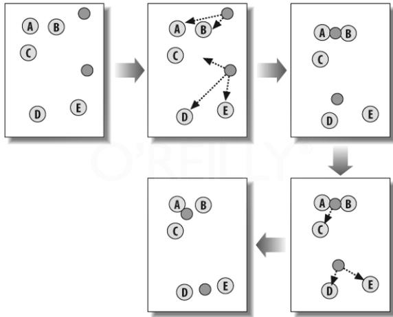
Figure 2: example of K-means algorithm execution
