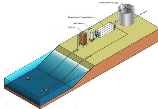
Figure 3: Osmosis water purification plant and detail of osmosis pressure vessel (<http://danolyte.com/it/progetti-speciali/desalinizzazione.html>)
