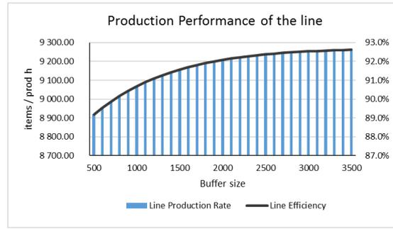
Figure 6: Production performance for different buffer sizes.
