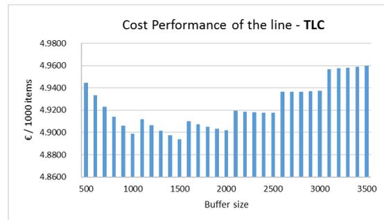
Figure 8: TLC values for different buffer sizes.
