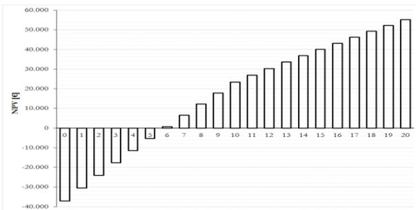
Figure 7: NPV of the geothermal system using groundwater; with the incentive
