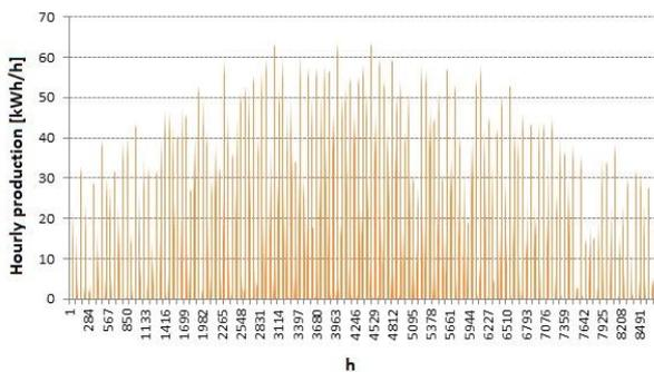
Figure 3: hourly production of the PV plant in a year
