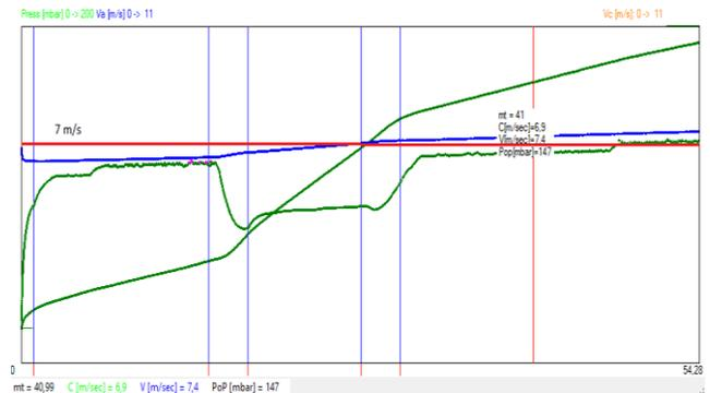
Figure 9: Simulation result by TPSim Win. Pressure loss (dark green line), solid velocity (green line) and air velocity (blue line) are plotted as a function of pipeline length, with a solid loading ratio  $m/m_{max} = 0.68$  and a duct internal diameter of 215 mm.
