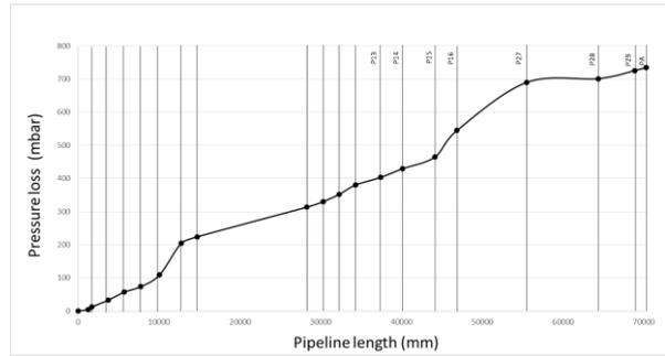
Figure 6: Pressure drop is plotted as a function of pipeline length.
