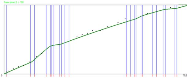
Figure 7: Pressure drop calculated by TPSim Win (green line) and experimental values (black points) are plotted as a function of pipeline length.
