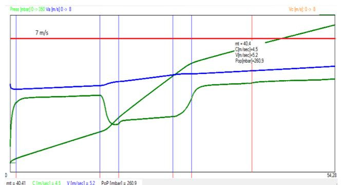
Figure 10: Simulation result by TPSim Win. Pressure loss (dark green line), solid velocity (green line) and air velocity (blue line) are plotted as a function of pipeline length, with a solid loading ratio  $m/m_{max} = 0.93$  and a duct internal diameter of 215 mm.
