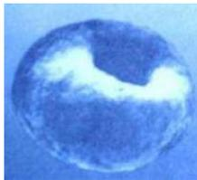
Figure 1: Enlargement 300:1 of atomized slip.
