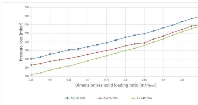
Figure 8: Total pressure loss  $\Delta p$  expressed as a function of dimensionless solid loading ratio  $m/m_{max}$  for different values of pipeline diameter size.
