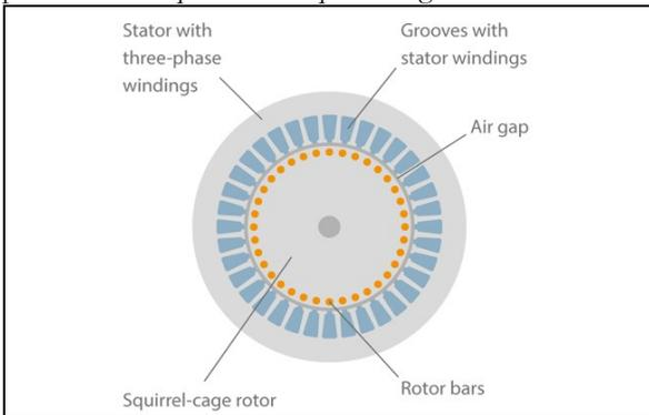
Figure 3: sectional view of an asynchronous motor
