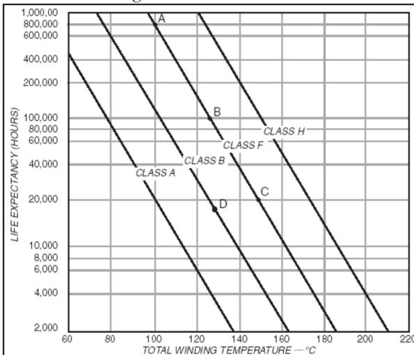
Figure 4: relationship between temperature and insulation life expectancy
