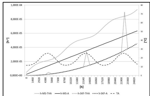
Figure 6: failure rate trends according SKF and Military standard methods with or without thermal aging
