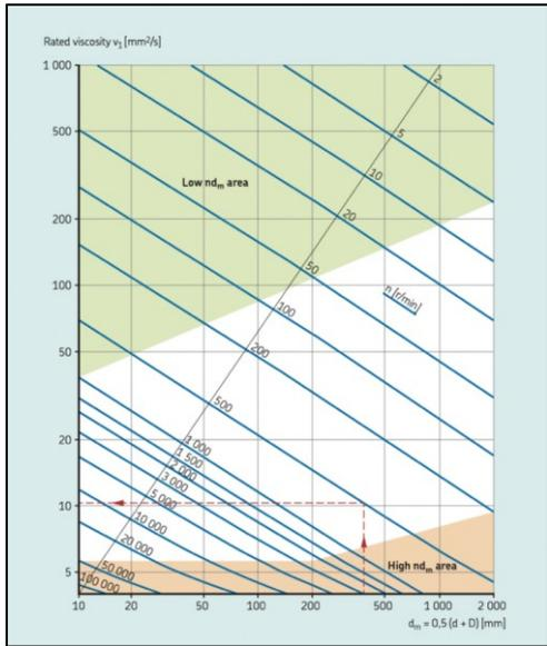
Figure A1: estimation of the rated viscosity  $\nu_1$
