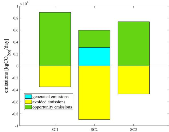
Fig 2. Predicted emissions in WWTP "Bari Ovest" for each scenario.
