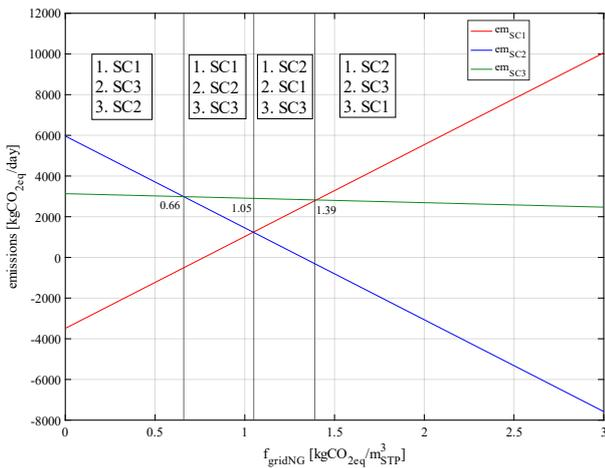
Fig 4. Trends of the emission functions by varying the emission factor from the gas grid for each scenario.
