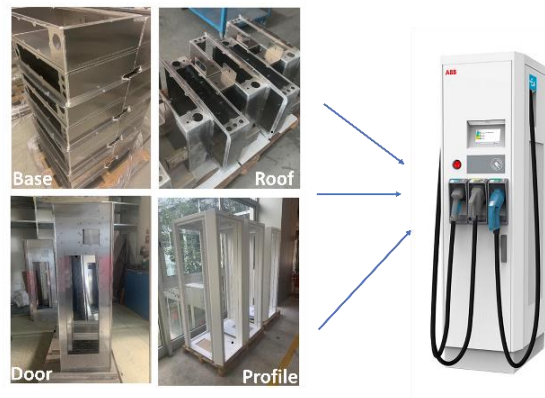
Fig.3. Cabinet TX and its elements
