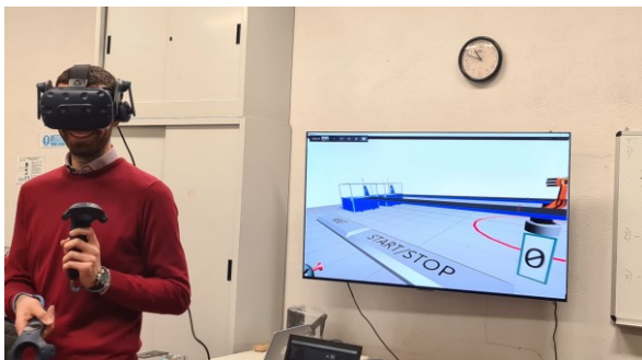
Figure 11. Photo from pilot testing: details of interactive buttons implemented to enable start and stop of the simulation inside the VR environment.
