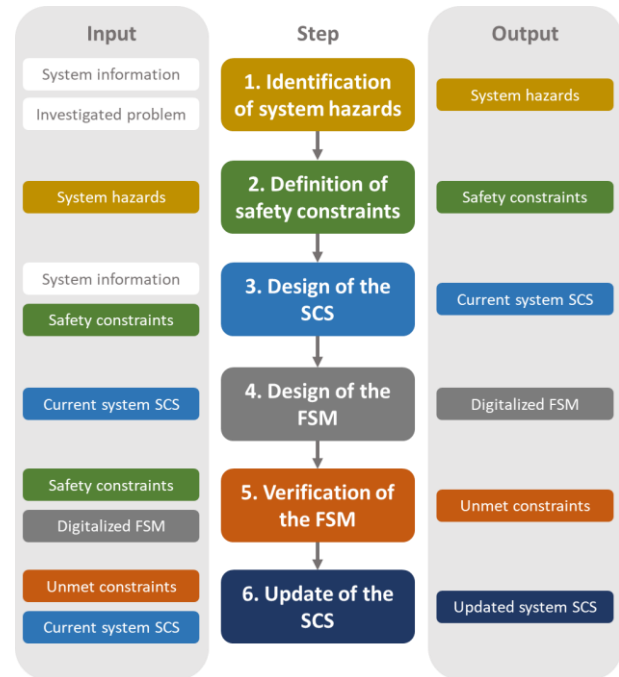
Fig. 1 Schematization of the proposed methodology to integrate STAMP and model checking. The color code relates input/output blocks with the corresponding methodology step. White blocks enter as pre-required input to apply the methodology.
