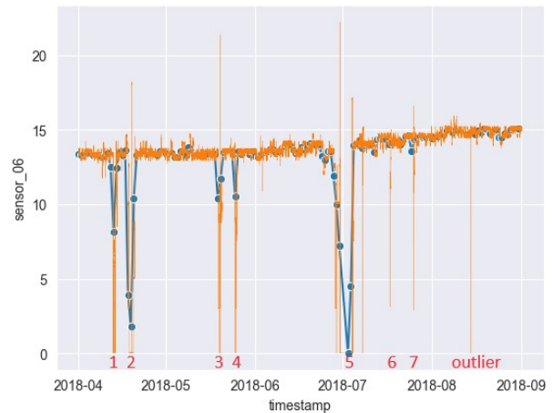
Figure 5 Line plot in orange and moving average plot in blue (The failures are numbered in red and the drop after 2018-08 is an outlier). The values are not normalized.
